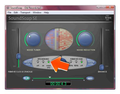
**5.** Adjust the Noise Reduction Knob. Next, adjust the Noise Reduction knob on the right. Turn the Broadband mode button to On and start playback again. This time, turn the Noise Reduction knob the minimum necessary to remove the background noise. If the material being cleaned is dialog, also click the Preserve Voice button at the left. This filter will automatically remove sounds outside of the range of human voices. Notice how the Wash Window, formerly mostly red, is now turning blue?
